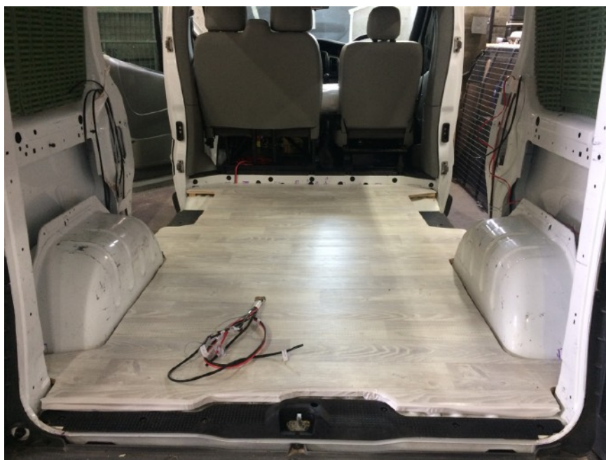
Figure 3. The floor. The wiring runs underneath in conduit. The vinyl is in place.
