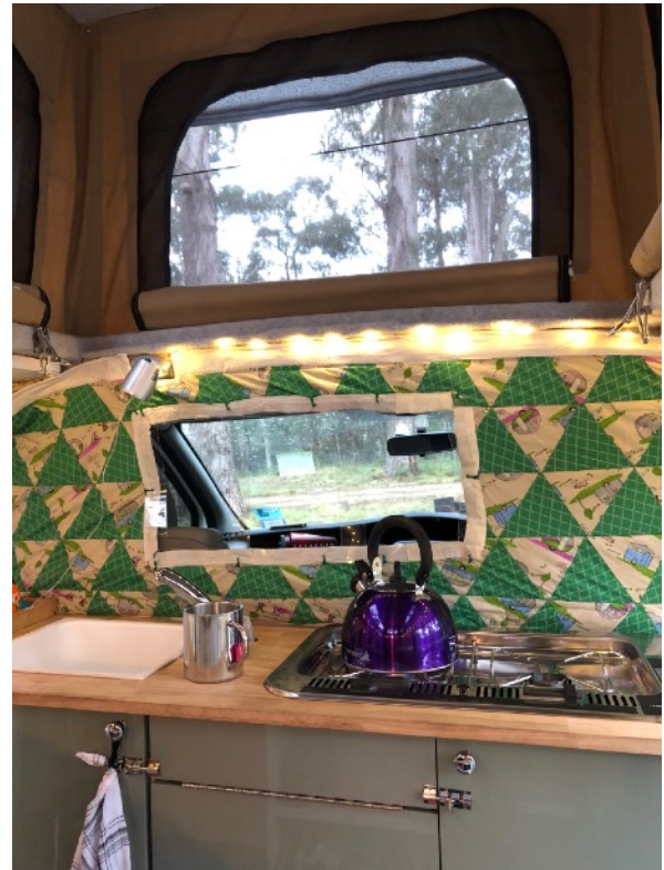
Figure 19. The finished campervan, interior. It has running water, solar-power, and a spirit stove.
