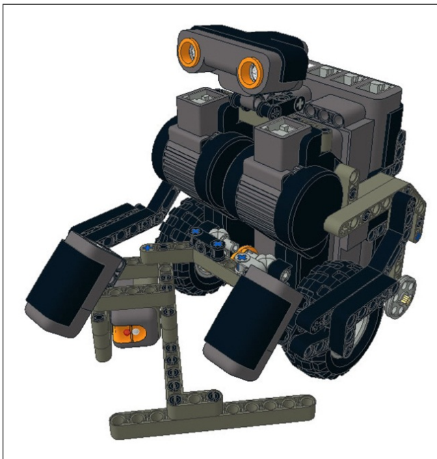
FIG. 1. Arturito, the brick-sorting Lego NXT robot.
