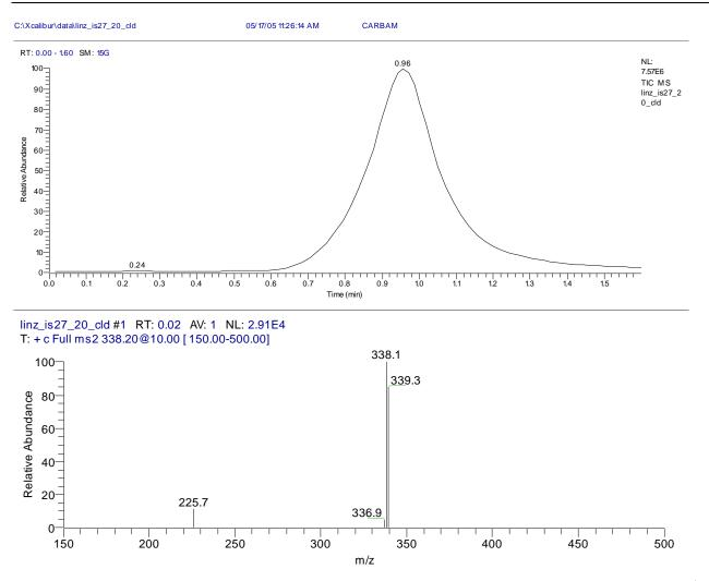
**Figure. 2b**.TIC chromatogram of a human plasma spiked with linezolid (Rt:0.96 min) as an internal standard (C:  $1 \mu gml^{-1}$ ) using +APCI-LC-MS (linezolid: m/z 338.1).
