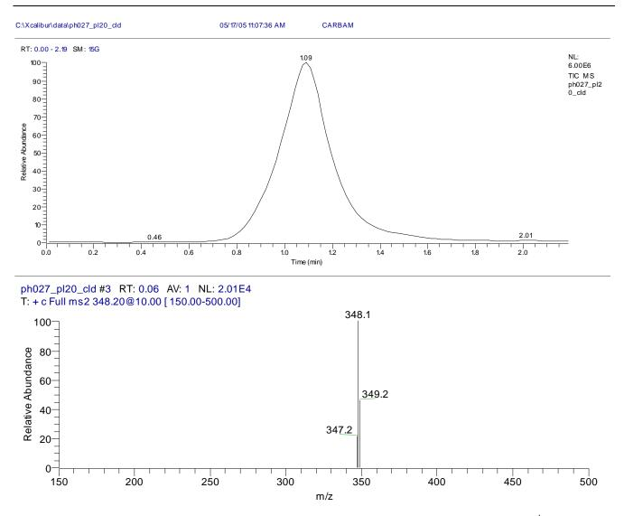
**Figure. 2a.** Representative TIC chromatogram of a human plasma spiked with PH-27 (Rt: 1.09 min) (C:  $5 \mu gml^{-1}$ ) using +APCI-LC-MS (PH-27: m/z 348.1).
