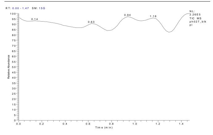
**Figure 3.** TIC chromatogram of a 50-µl aliquot of free human plasma (Blank) after treatment with acetonitrile, using +APCI-LC-MS.
