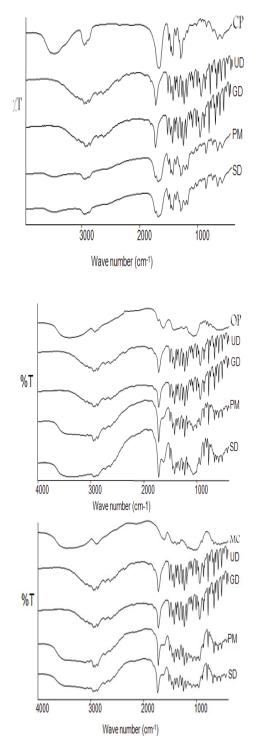
**Figure 4.** Fourier transform infra red spectra of the carriers crospovidone (CP), oleaster powder (OP) and microcrystalline cellulose (MC) together with those of unground drug (UD), ground drug (GD), physical mixtures (PMs) and solid dispersions (SDs) of the carrier: drug ratio of 2:1.
