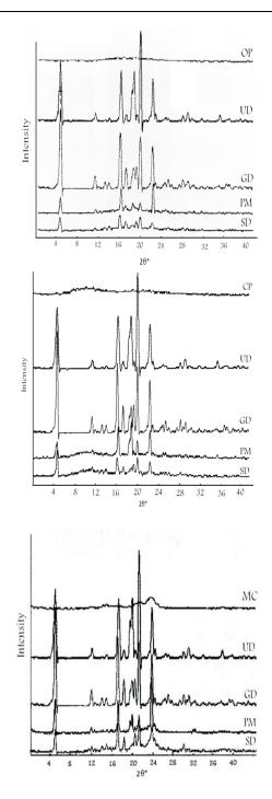
**Figure 3.** Powder X-ray diffraction pattern of the carriers crospovidone (CP), oleaster powder (OP) and microcrystalline cellulose (MC) together with those of unground drug (UD), ground drug (GD), physical mixtures (PMs) and solid dispersions (SDs) of the carrier: drug ratio of 2:1. its integration in terms of dw as well as dM between times 0 and t gives:
