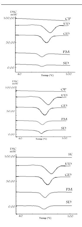
**Figure 2.** DSC thermograms of the carriers crospovidone (CP), oleaster powder (OP) and microcrystalline cellulose (MC) together with those of unground drug (UD), ground drug (GD), physical mixtures (PMs) and solid dispersions (SDs) of the carrier: drug ratio of 2:1
