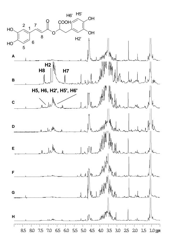
**Figure 1.** 500MHz <sup>1</sup>H NMR spectra of commercial tinctures (A-H) derived from fresh and dried *Melissa officinalis*.
