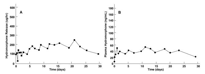
**Figure 6.** (A) In-vitro release of hydromorphone from coated polymer disk with a central uncoated channel and (B) plasma hydromorphone concentrations in rabbits after subcutaneous implantation of the polymer disk (adapted from reference 4)
