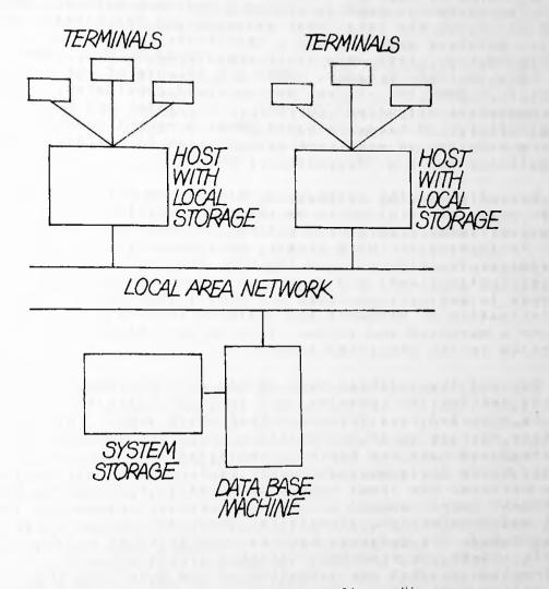
Figure 1: The System Configuration
