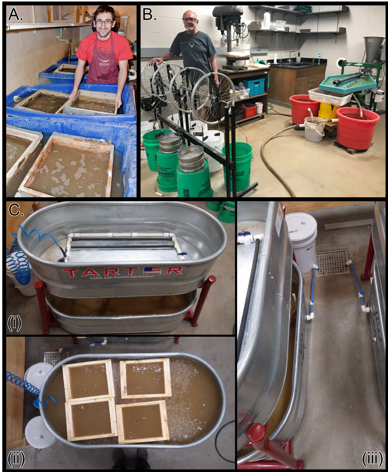
Figure 1. Examples of novel institutional-based bulk matrix processing setups. A, the soaking tank station at the Royal Tyrrell Museum of Palaeontology (RTMP). While the water can be drained from each large tank, the screenboxes float at the surface and are processed essentially following the same techniques and procedures implemented as if in the field. Photo of technician C. Capobianco with the RTMP's screenwashing station provided by T. Cullen. B, the motorized bike wheel setup in the lab of R. Rogers at Macalester College. This motorized construct entails the rotation of each wheel which raises and lowers each of the sediment-laden sieves within a bucket of water – analogous to the raising/lowering of a tea bag. Photo courtesy of R. Rogers and Macalester College. C, (i-iii) Soaking tanks at the North Dakota Heritage Center & State Museum that use a pneumatic line for aqueous agitation. Note that water in the top tank can drain to the lower tank, and from there wastewater is piped from each tank station to a drain. Photos courtesy of C. Boyd and the North Dakota Geological Survey.
